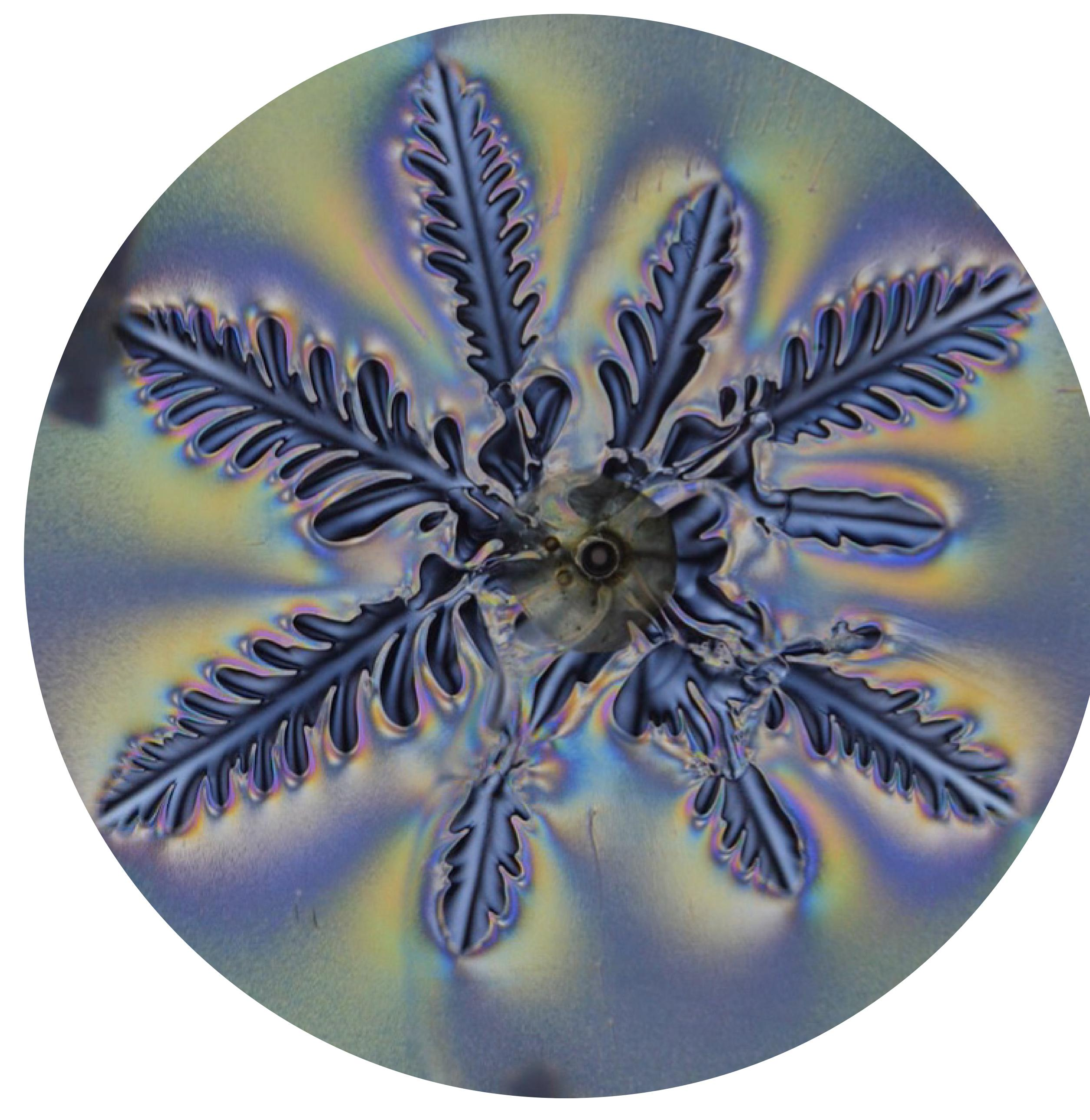
The displacement of a liquid crystal by a less viscous silicone oil in a Hele-Shaw cell leads to an instability.
